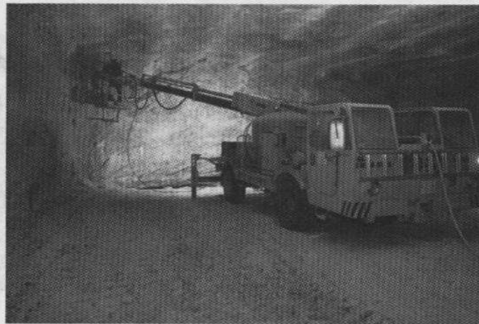
Fig. 4: Blasting vehicle with lifting platform
